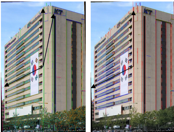
Figure 4: Vanishing points estimation results on a picture from test set: left– results obtained by method proposed in [1], right– results of our method
