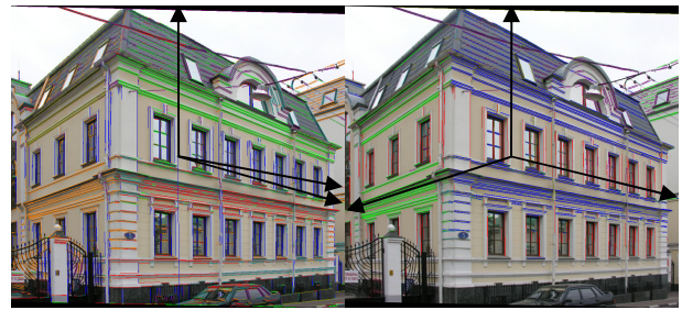
Figure 5: Vanishing points estimation results on a picture from test set: left – results obtained by method proposed in [1], right – results of our method
