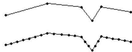
Figure 3: Input polyline (top) and splitted polyline (bottom).
