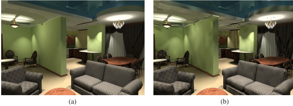
Figure 7: Example animation frames (a) with and (b) without temporal processing for about 80,000 photons per frame. An animation segment length of 31 frames was considered for the temporal photon processing. The average time of the indirect lighting computation per frame was less than 3 seconds.
