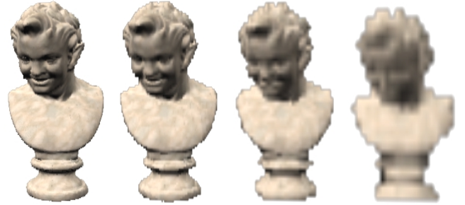
Figure 20. Textured LODs obtained by relief texture mapping the first four levels of a relief texture map pyramid. Relief texture resolution: 256x256 texels (left) down to 32x32 texels (right).
