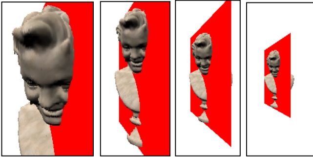
Figure 19. Depth-correction using 8-bit quantized \Delta z values.
