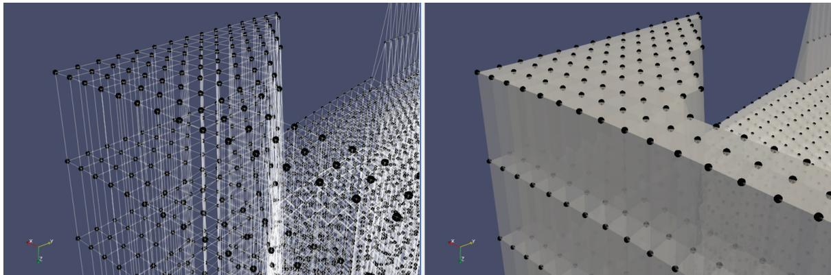
**Figure 6:** Edges and faces of unstructured grid cells with duplicated points
