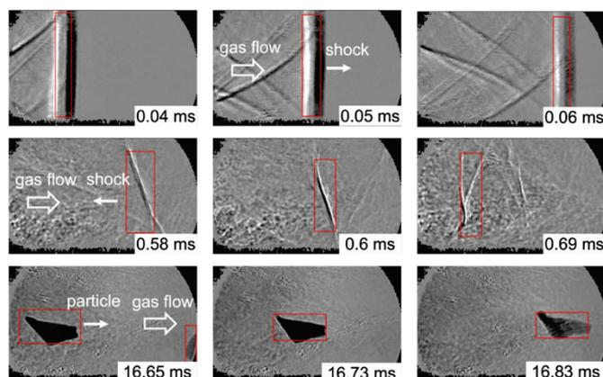
**Figure 5:** Flow structures detection on the shadowgraph images of the flow in shock tube by CNN. First row – initial shock wave; second row – reflected discontinuities; third row – detection of parts of the destroyed diaphragm
