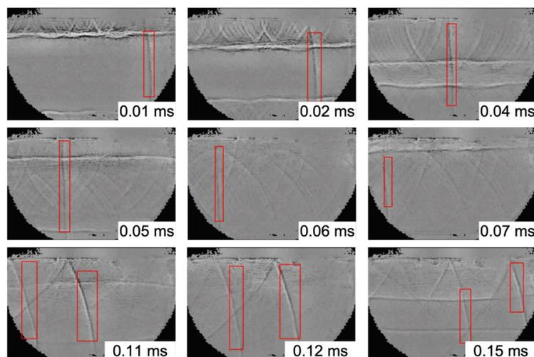
**Figure 8:** Flow structures detection on the shadowgraph images of the complex post-discharge flow by CNN
