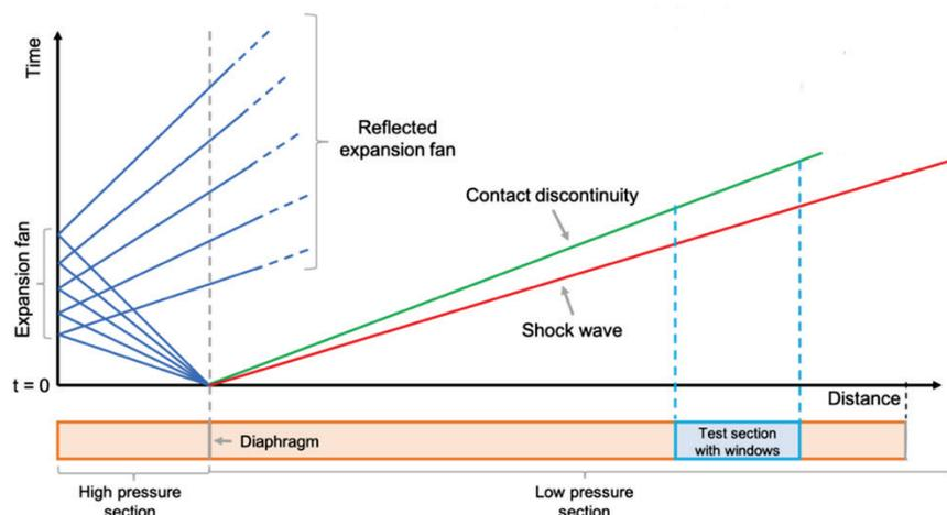
**Figure 2:** Shock tube scheme and x-t plot of gas flow development after diaphragm rupture
