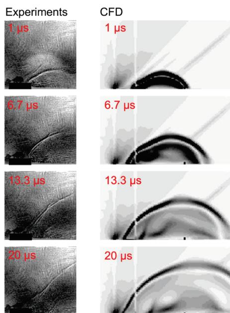
**Figure 3:** Shock wave spreading from the pulsed surface electrical discharge in the supersonic flow near the obstacle: CFD and experimental shadowgraph images comparison
