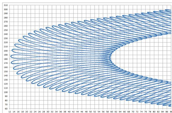
**Figure 1:** Sun position in the hemisphere during a year; azimuth is vertical and polar angle is horizontal
