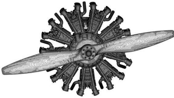
Figure 13: Engine model wrapping, constructed in 48 minutes and 44 seconds on core i5-3450 CPU.
