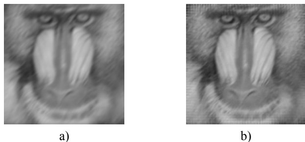
Figure 3. Blurred image baboon ( \alpha = 45, L = 8, W = 3 ): (a); image restored using total variation deblurring [14] (b).
