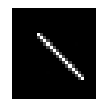
Figure 1. An illustration of the PSF function (1), corresponded to \alpha = 45, L = 15 . The contrast of the image was increased.
