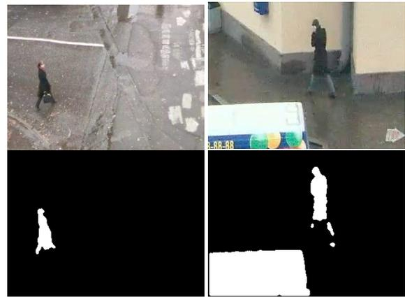
Fig. 4. Examples of background subtraction using proposed algorithm.
