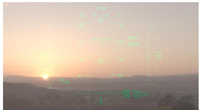
Fig. 7. An example of AR image synthesis for the environment with a high level of luminance.
