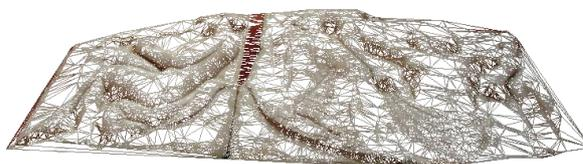
Figure 2: Triangulation for a part of bas-relief
