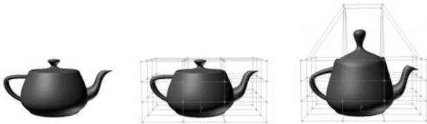
Figure 2: Example of a FFD applied on a teapot. Middle image, the teapot is embedded in a parallelepipedal mesh. Right, deforming the embedding volume implies the deformation of the teapot.
