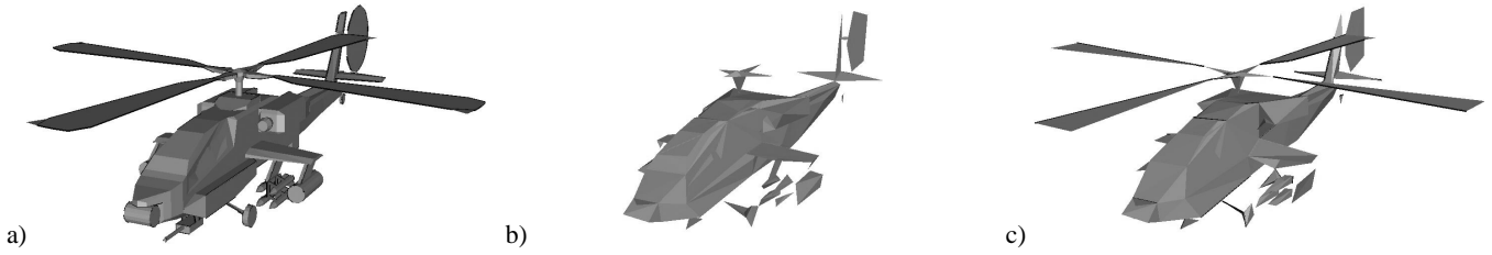
Figure 1: Simplification with and without feature preservation: a) original model (1972 vertices); b) reduced to 200 vertices without feature preservation; c) reduced to 200 vertices with features preserved.
