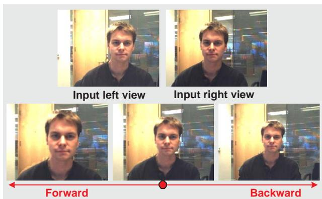
**Figure 6: Forward/backward translation of virtual camera.** The bottom row shows the synthesized cyclopean views with (left) forward virtual camera translation, (centre) no virtual camera translation, (right) backward virtual camera translation. Notice the *parallax* effect around the head.
