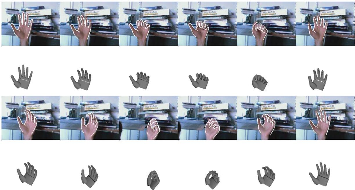
Figure 13: **Tracking a hand opening and closing with rigid body motion in front of clutter.** In this sequence 6 DOF for rigid body motion plus 2 DOF for finger flexion and extension are tracked successfully.
