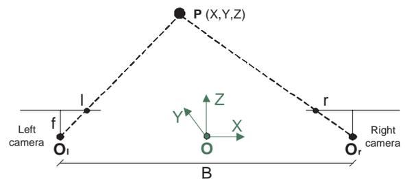
**Figure 10: Basic camera configuration and notation.**  $O_l$  and  $O_r$  are the optical centres of left and right cameras respectively,  $f$  is the focal length of the cameras (identical for both cameras) and  $B$  is the baseline between the two optical centres. The origin of the reference coordinate system  $X, Y, Z$  is denoted  $O$ .
