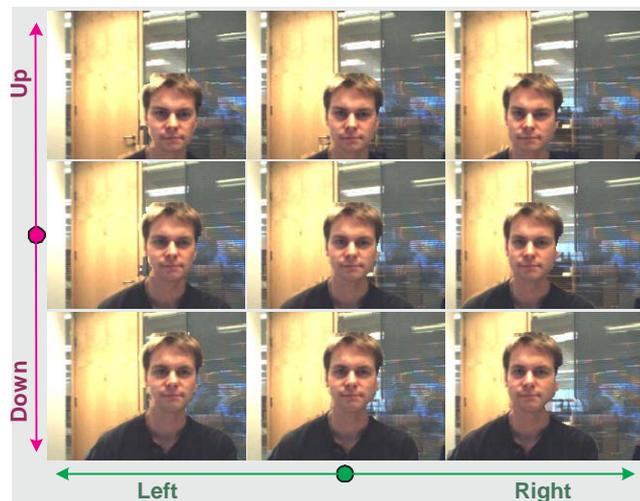
**Figure 7: In-plane translation of virtual camera.** The left and right input images are the same as in fig. 6. This table shows the synthesized images corresponding to translation of the virtual camera along the  $x$  and  $y$  axes. Notice the *parallax* effect around the head. Also, the door frame is reconstructed nicely despite it being partially occluded in the right input view.
